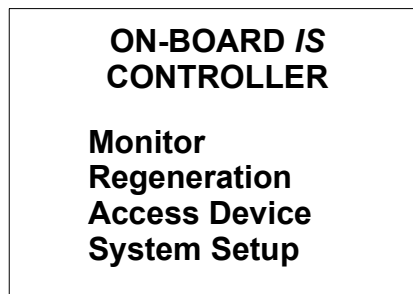
Figure 4-1: On-Board IS Controller Main Screen
